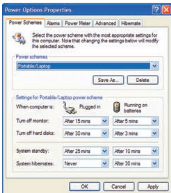
The power-saving settings window of a Windows XP laptop: Start / Control Panel / Power Options.
