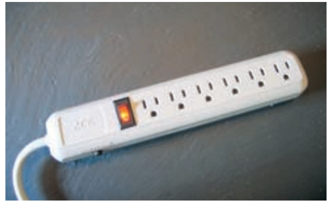
A switched plug strip makes it easy to power-down peripherals and phantom loads.
